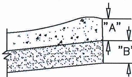
"A" CONCRETE/ BITUMINOUS
